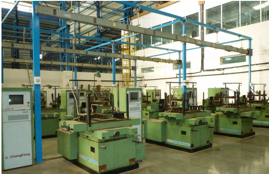
EDM wire cut machines for split master link machining
