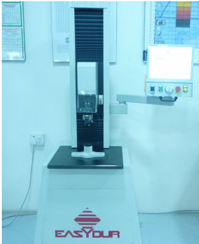
Universal hardness testing - Rockwell, Vickers & Brinell
